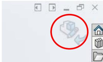
**Figure 8.** The icon in the top-right corner of the graphics area for returning to assembly.
